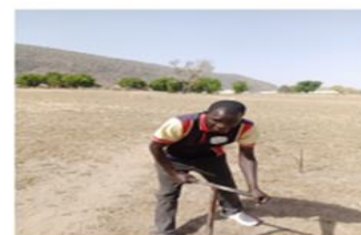
Plate 3: Auguring the soil for disturbed soil sample.
